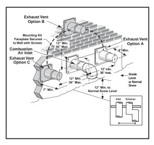
Figure 19. Exhaust and Combustion Air Pipe Clearances
